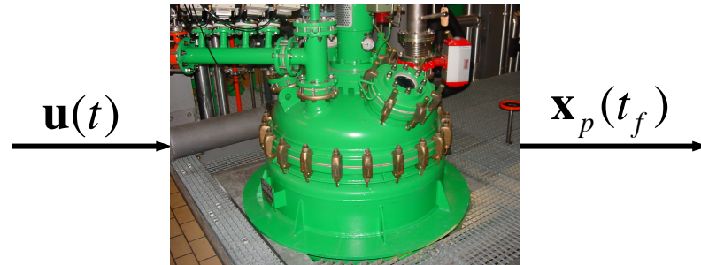
Batch reactor with finite terminal time
